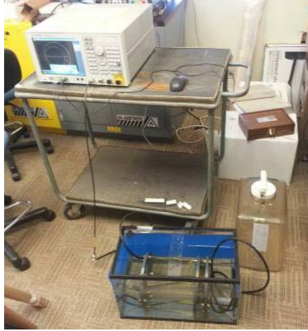
Figure 6. Experimental setup for two-coil measurements in a seawater tank.
