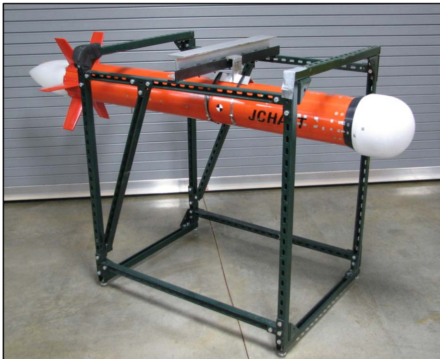
Figure 7. JCHAAT Tow Swing Setup
