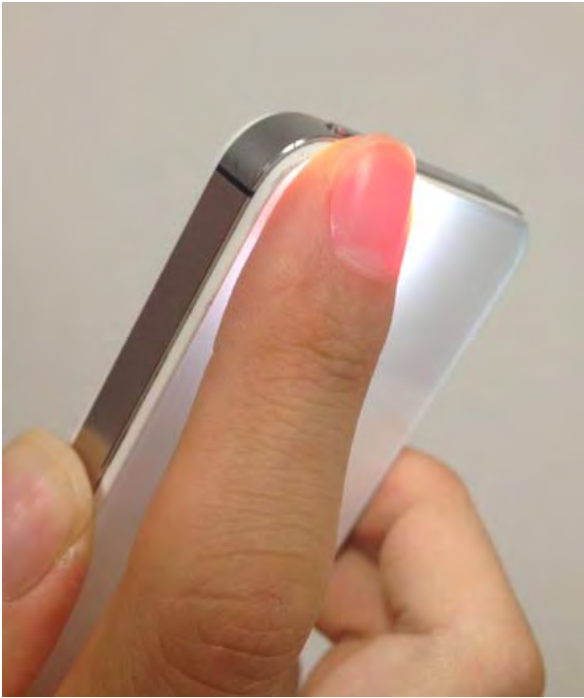
Fig. 1. A smart phone application for data recording (the application uses the camera lens and illumination to acquire information about heart rate and rhythm).
