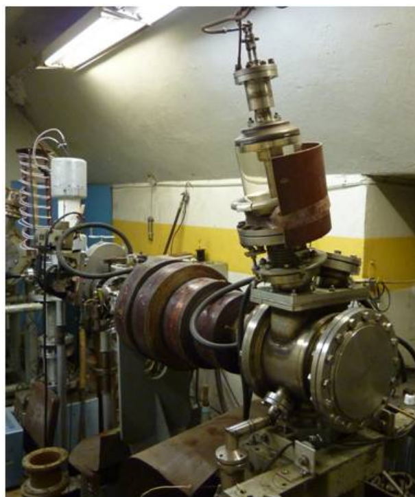
Figure 4. Appearance of the device (above), complete view of the device (below), electron source with the beam transport system
