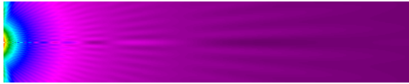
Figure 118. Spherically Spreading Beam Field Of Point Source By Using F-K Model Via Equation (1)
