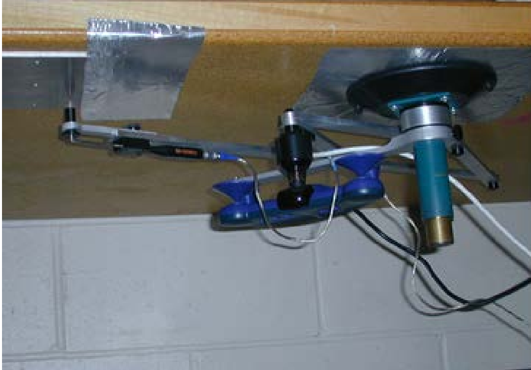
Figure 136. Inverted Tests Of Pantograph Scanner To Evaluate Rigidity Of Linkages And Ability To Support Probes And Cabling So To Eliminate Liftoff Of The Probes And Minimize Operator Fatigue
