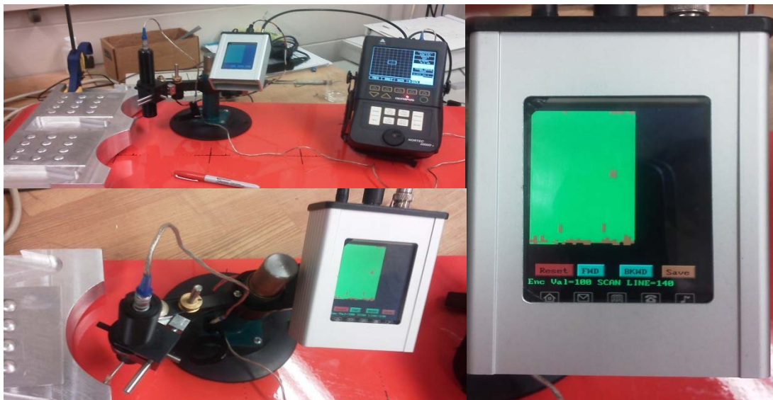
Figure 139. Testing Of The Arc Scanner, With Zoom Of LCD Screen Showing EDM Notch Indications And Edge/Liftoff Effects At Top And Bottom Of Image Corresponding To The Edges Of The Arc Section On The Mockup Panel
