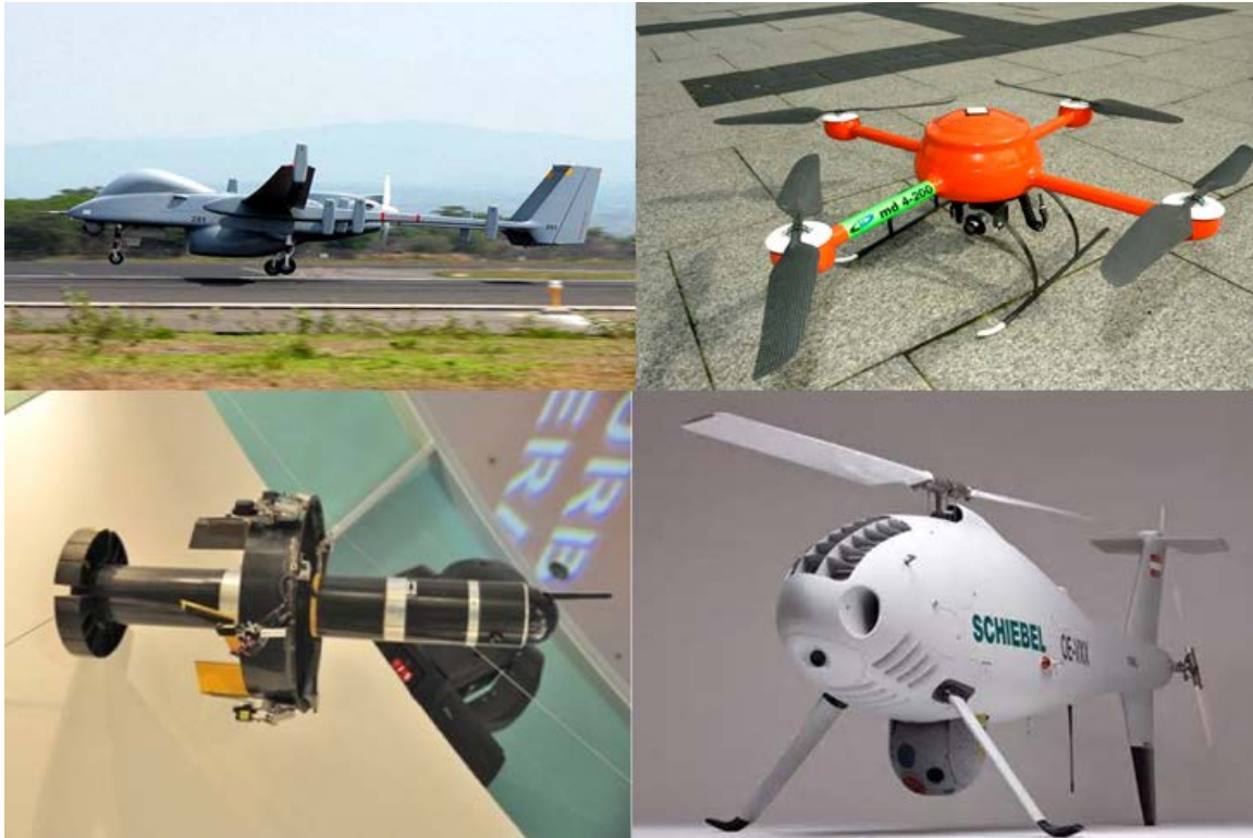
Figure 4. Example of fixed wing, quadrotor, helicopter and other hybrid forms of UAVs (clockwise from top left). From [33–36].
