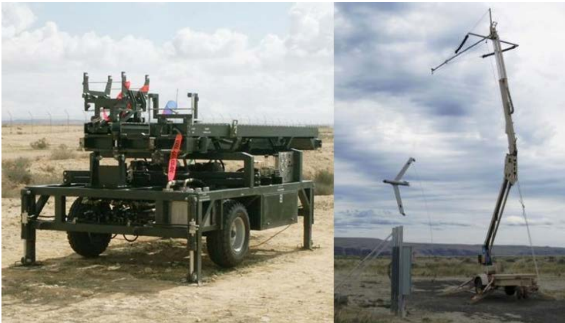
Figure 6. Example of UAV Launch System and UAV Recovery System (left to right). After [40] and [41].
