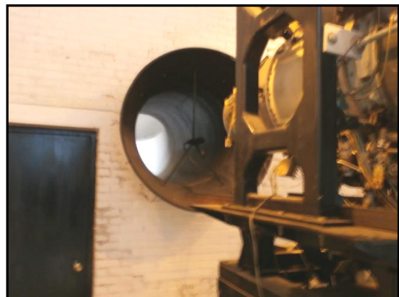
Figure 8. F-109 Turbofan Emissions Probe in Exhaust Duct
