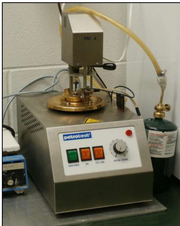
Figure 20. Petrotest PM-4 Flashpoint Tester
