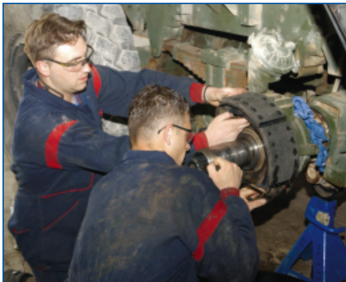
Two Kosovars replace brakes on an M978 heavy, expanded-mobility, tactical truck. Local nationals work with the Kosovo Force to keep vehicles and equipment operational.
