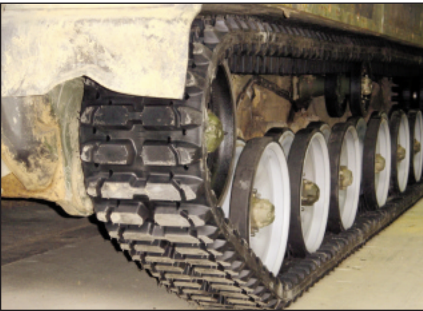
The band tracks on this M2A2 Bradley fighting vehicle yield a smoother, quieter ride.
