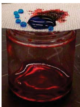
Superhydrophobic/oleophilic dip-coated fabric Tuteja et al , Science, 2007 , 318, 1618
