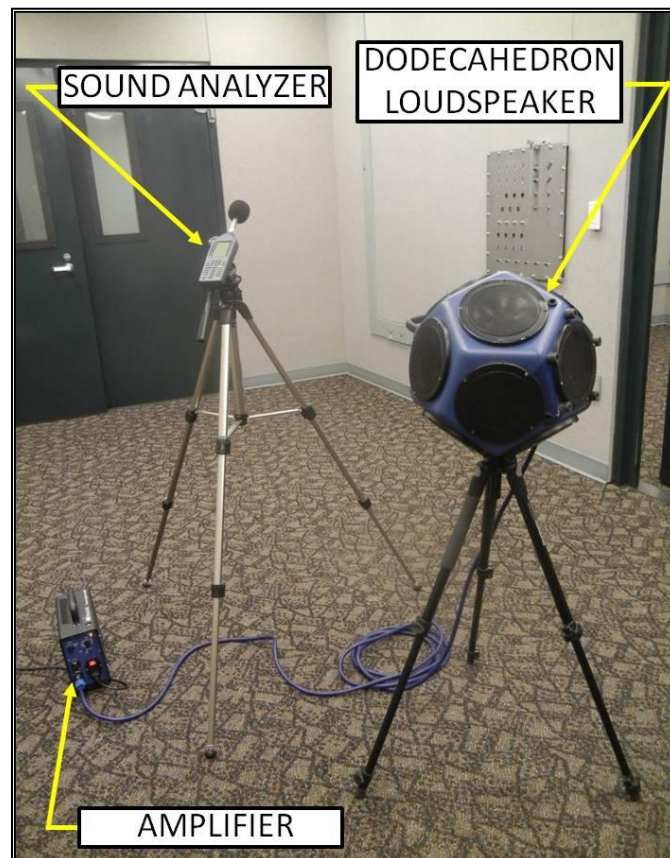
Figure 15. MIND Laboratory: typical instrumentation for acoustic testing.
