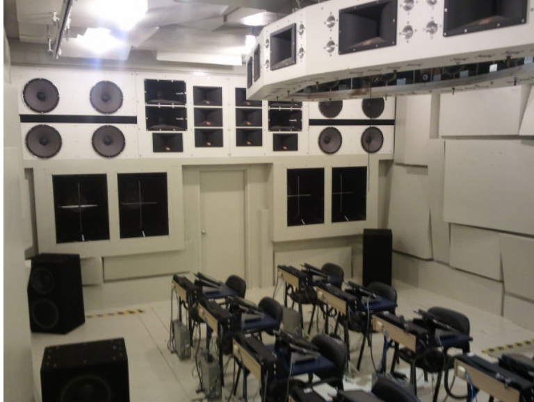
Figure 6. AFRL's VOCRES facility used to measure speech intelligibility performance
