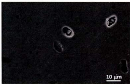
Figure 2. SEM (SE) image of \text{ZrW}_2\text{O}_8 pellets sintered at 1175 °C for 1 h.
