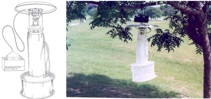
Figure 7. Illustration of SSAM trap with collection net and deployed.
