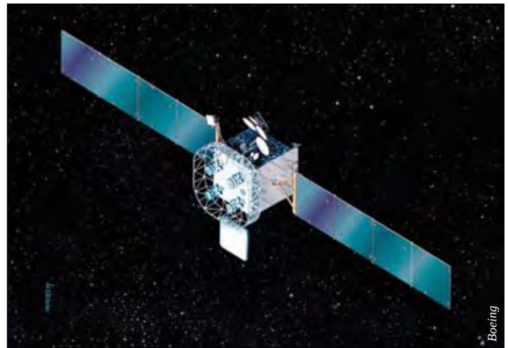
Global Broadcast Service (GBS) payload host: Ultra-high Frequency Follow-on (UFO) satellite.
