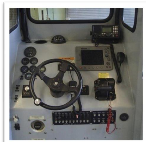
Figure 4.25.3 Console and Transponder
