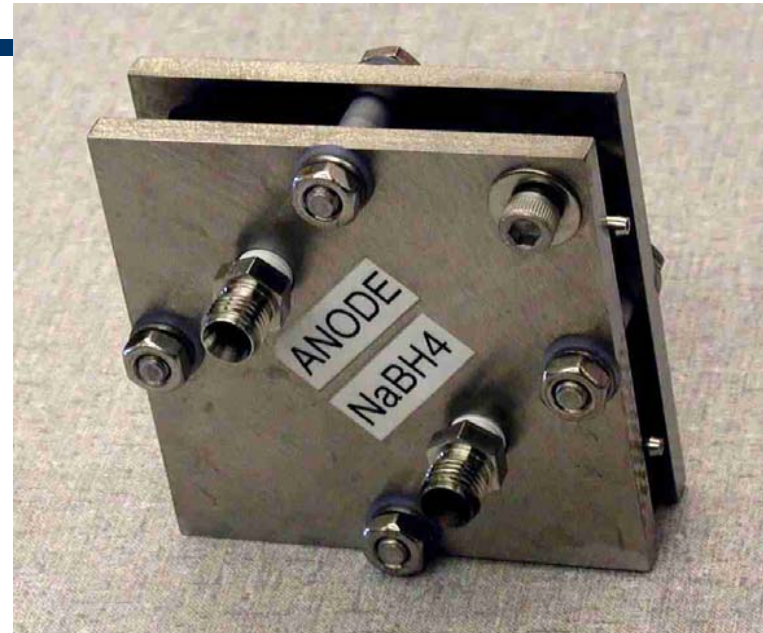
15-W NaBH 4 /H 2 O 2 Test Fuel Cell as assembled.
