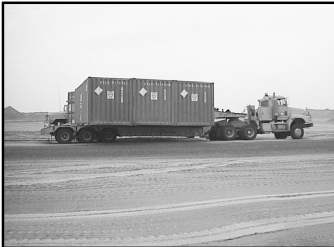
Alpha Company, 62d Engineer Battalion, transports pipe by loading three MILVANs on a lowboy.
