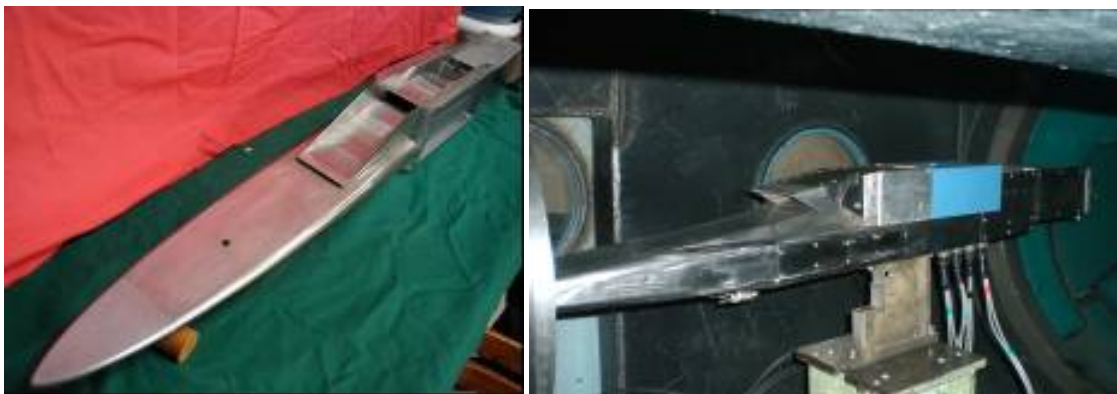
Figure 9: Forebody/air inlet tested in the Mach number range 2 to 4.
