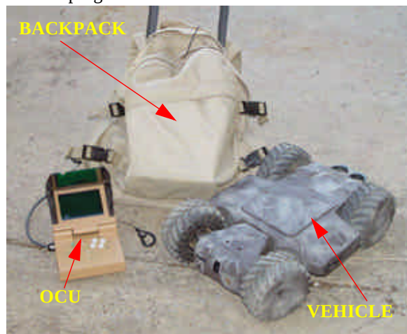
Figure 1 : Dragon Runner System: Vehicle & OCU
