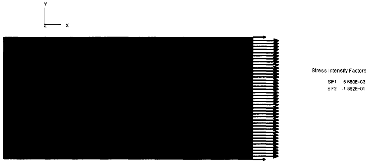
Figure 13: Finite Element Plate Model Showing Crack Growth of 70 mm
