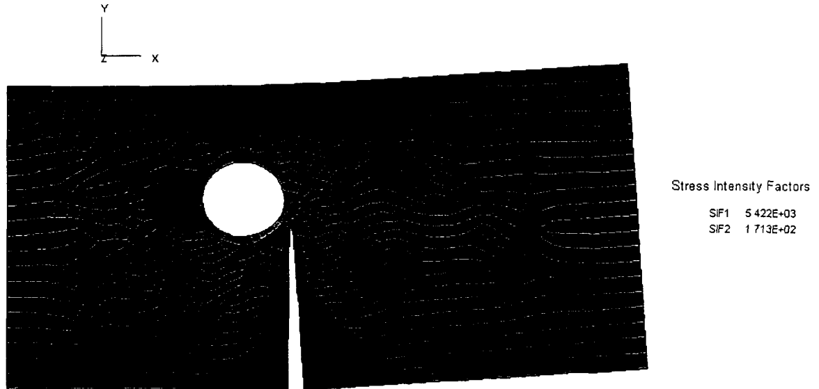
Figure 23: Crack Turning in the Plate Model with a Hole Under Mode I Loading
