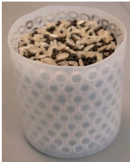
FIG. 1. The scanning container filled with 50% weight of spheres to ellipsoids. Note the hemispherical beads on the boundary of the container used to minimize boundary effects.
