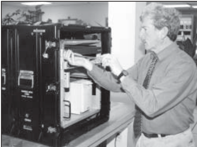
Figure 22. Dennis Green, a mechanical engineer in Tobyhanna Army Depot’s Satellite Communications System Directorate, attaches a component of a communications transit case designed for Special Forces. The case allows soldiers to communicate via satellite terminals.
