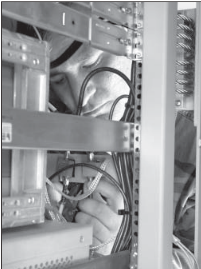
Figure 16. SPC Mayo Vandyck from 40th Signal Battalion ensures cables are tight during the power-balancing procedure before operating equipment in the Transportable Theater Injector. The TTI provides the satellite connection for the Theater Injection Point, the new communications equipment 11th Signal Brigade soldiers are training to operate.
