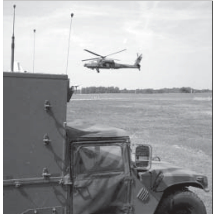
Figure 25. Fort Campbell's proof-of-concept demonstration tested EIS+ on both helicopters and humvees. Part of EIS+ is the MT2011 transceiver, seen as a small white box on top of the humvee.
