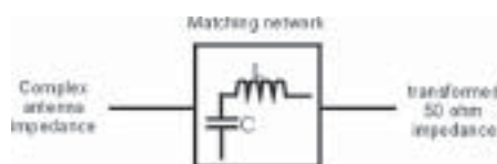
Figure 38. The network transforms the antenna’s complex impedance into a 50-ohm resistive impedance.
