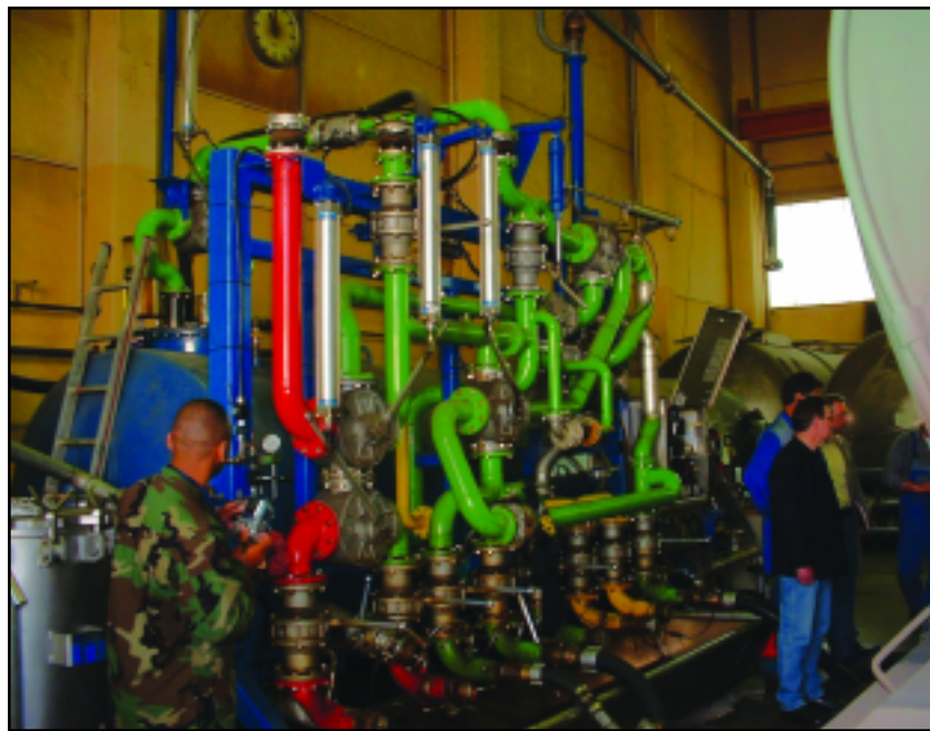
This hydrostatic test apparatus is used to test Army tankers at Industriewerke Saar GmbH.
