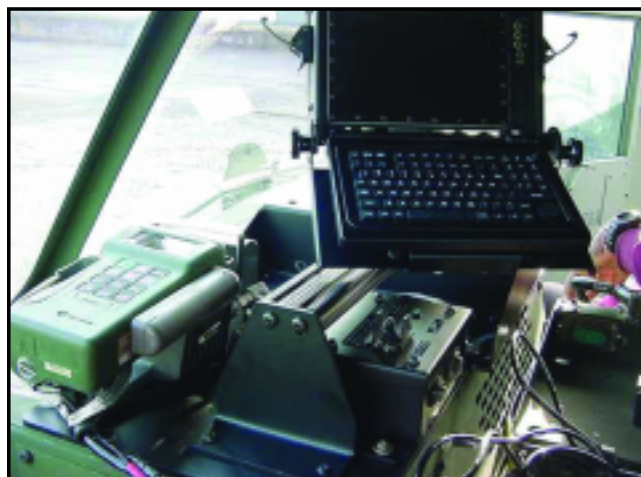
An MTS computer system is mounted on the dashboard of a heavy, expanded-mobility, tactical truck (HEMTT) (above). The computer slides into a mounting station that is installed on the HEMTT's dashboard (below).
