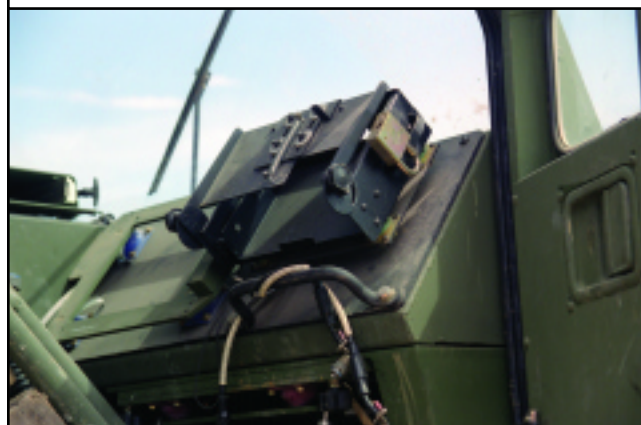
An MTS computer system is mounted on the dashboard of a heavy, expanded-mobility, tactical truck (HEMTT) (above). The computer slides into a mounting station that is installed on the HEMTT's dashboard (below).
