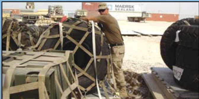
A soldier uses a 10,000-pound Atlas forklift to place a 463L pallet onto a trailer for transport. (Inset) A soldier secures the load on a 463L pallet.
