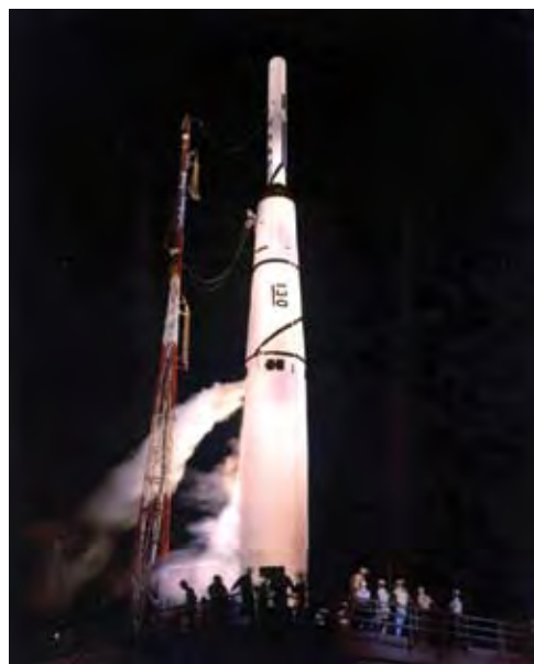
Thor 130 stands on the pad on 11 October 1958, holding the Pioneer 1 payload. Although the fourth stage traveled about 70,717 statute miles into space, its trajectory was slightly off, and it did not quite achieve escape velocity despite firing all eight of the fourth stage solid rockets.
