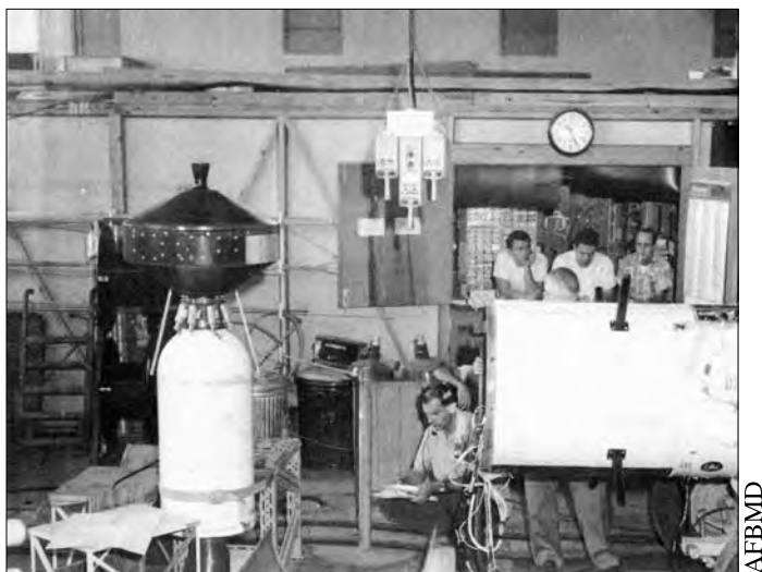
This photograph shows the interior of STL's testing lab in its hangar at LAX. Testing of the second, third, and fourth stages, probably for Pioneer 1, is under way. The top part of the Able second stage is visible at right on the wheeled vehicle. The spacecraft and fourth stage are mounted on the third stage at left. (Illustration from AFBMD, "Space Probes Program Status Report," 10 December 1958, figure 5)
