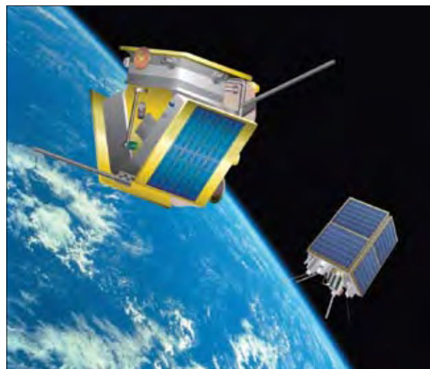
Fig. 3: Tsinghua-1, China's first microsatellite, observed by a Surrey Satellite Technology Ltd. (SSTL) microsat during proximity operations following a June 2000 launch. China has heavily leveraged its partnership with SSTL to advance its ability to field micro- and nano- class vehicles.
