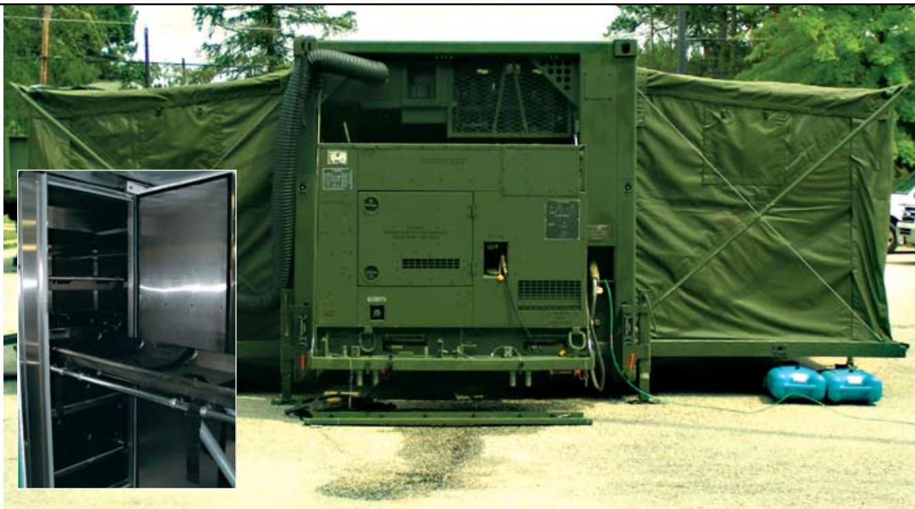
The environmentally controlled MIRCS system is self-sustainable for 24 to 72 hours and features a refrigerated remains storage compartment (inset) that can continuously cool 16 remains. Technicians can use this height-adjustable gurney to retrieve remains from storage.
