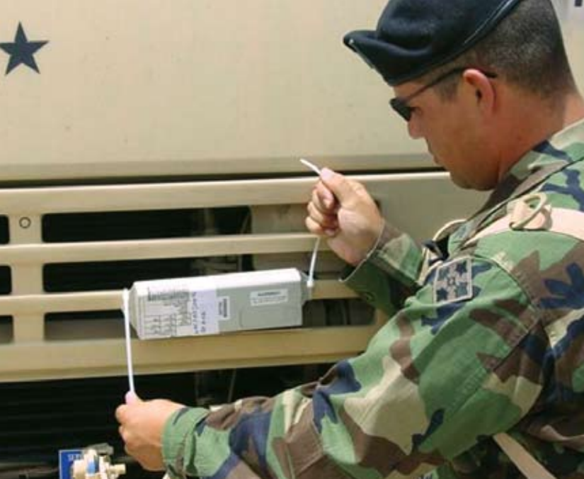
A Fort Carson, Colorado, Soldier attaches a radio frequency identification tag to a vehicle in preparation for a unit deployment.
