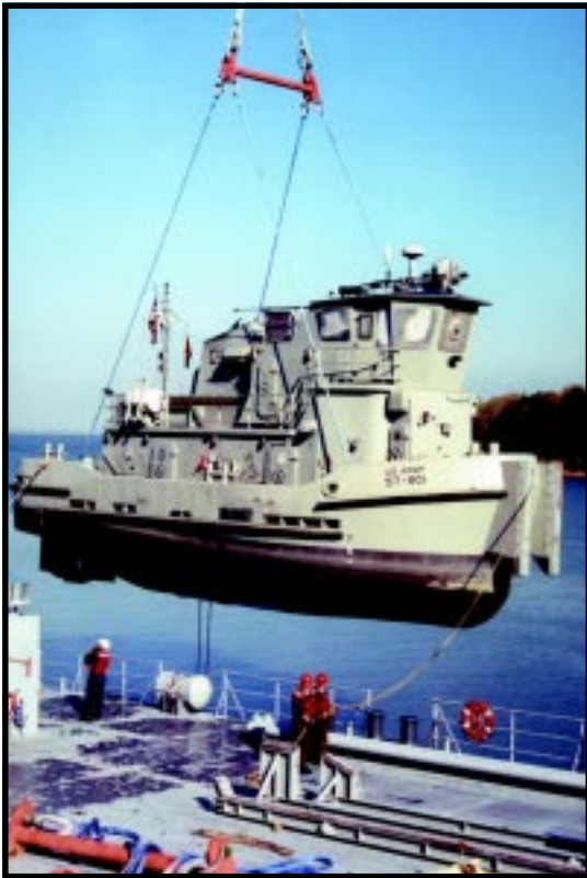
□ A tugboat is lowered onto the deck of the Army LSV.
