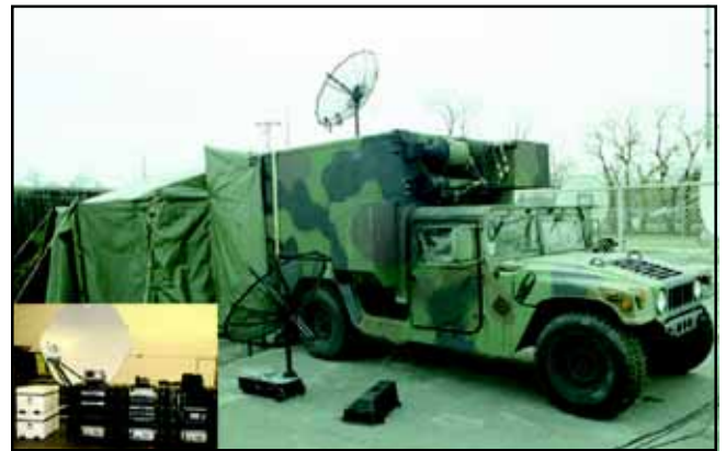
□ Pictured above is a mobile port operations center (MPOC), which includes a high-mobility, multi-purpose, wheeled vehicle (HMMWV) and a tent housing the Multimedia Communications System (MMCS, inset).
