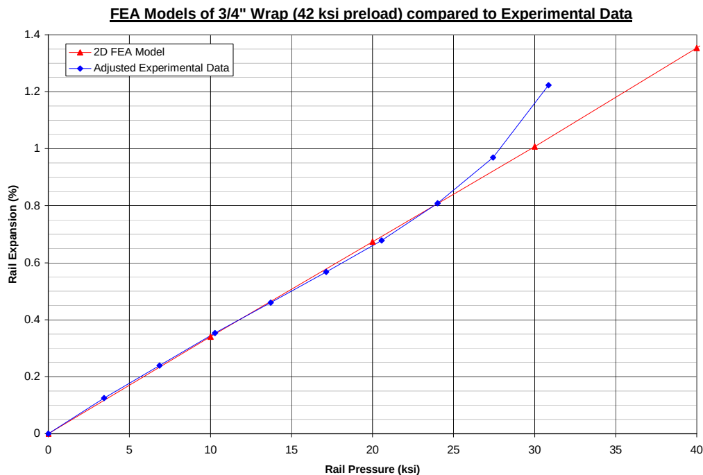
Figure 4. Comparison of FEA and adjusted experimental data (Cu rails)
