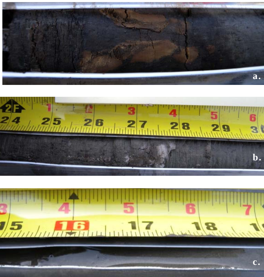
Figure 17. Sample cores from a depth of approximately 5 m (16.4 ft) at a) P1 (frozen), b) P5 (frozen), and c) at P6 (unfrozen and very wet).
