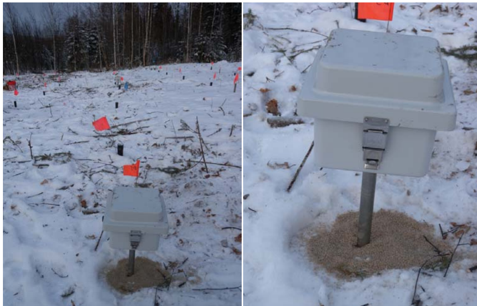
Figure 9. Example of 2 m long thermocouple string housing (TCP1-TCP4).
