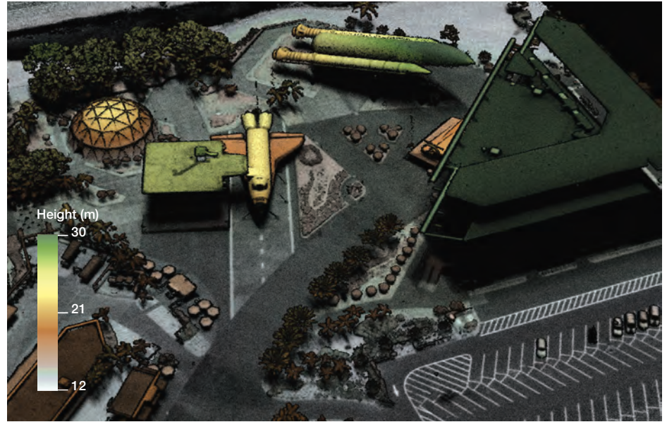
The 3D imagery of the Space Shuttle Explorer at the Kennedy Space Center complex in Florida was created from data acquired by the Airborne Ladar Imaging Research Testbed (ALIRT) system, shown at left.
