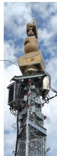
The Wide-area Infrared System for Persistent 360° Surveillance provides situational awareness in support of force protection applications. The sensor shown at left is secured inside a housing that is then mounted on a tower for surveillance applications.
