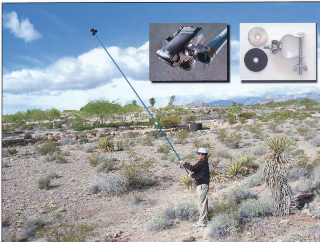
Figure 3-1. Example of hardware mounting bolts and hand-held swimming-pool skimming pole for taking aerial pictures.
