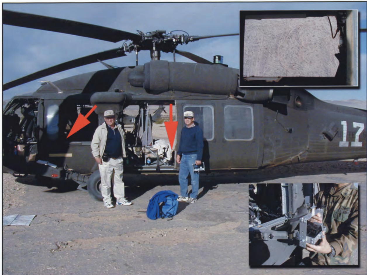
Figure 3-3. Blackhawk helicopter showing the location of two-camera mounting positions, side gun mount (left red arrow, lower right inset picture) and inside cargo hook door (right red arrow, upper right inset picture).
