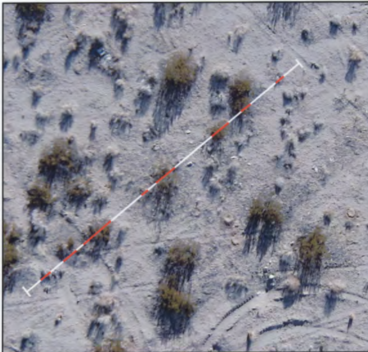
Figure 2-1. An example of a line intercept in Mojave Desert vegetation. The white line represents the measuring tape. The red lines indicate the portions of the tape that intercept shrub canopy. The percent shrub cover is the total length of the red divided by the white.
