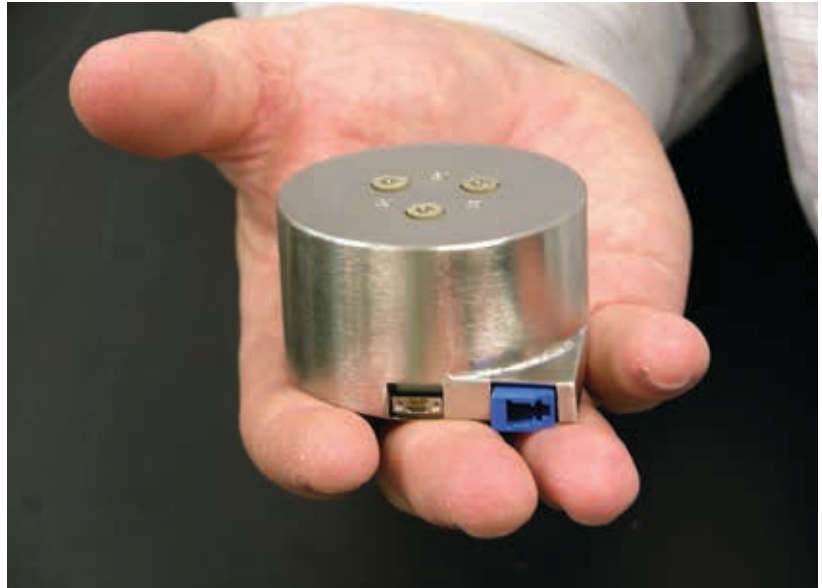
This commercial interferometric fiber-optic gyroscope is being characterized for use as an inertial sensor to be mounted on lasercom terminals to enable extremely stable pointing for acquisition and tracking.
