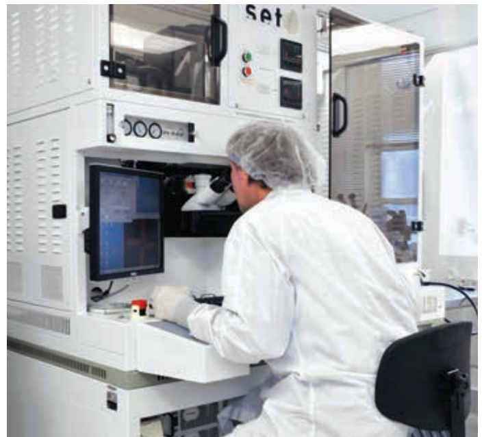
Al Ruff is operating a flip-chip bonding tool that is used to align and attach Geiger-mode avalanche photodiodes (APD) to readout integrated circuits (ROIC). An example of a dual 128 × 32 APD/ROIC integrated module is shown left.
