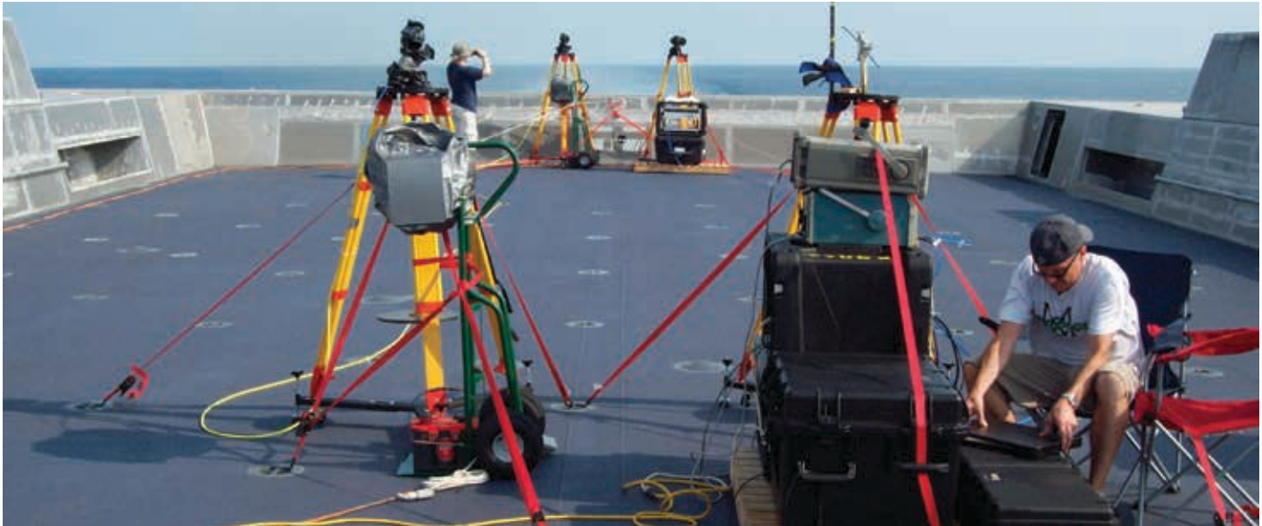
Staff members are deploying ship-based signal sources as part of the Laboratory's work evaluating surveillance radar performance in maritime environments.
