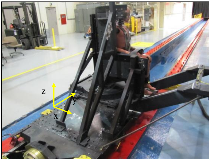
Figure 2a and 2b: HIA Facility Set-up for Lateral +Y-axis Impact Test
