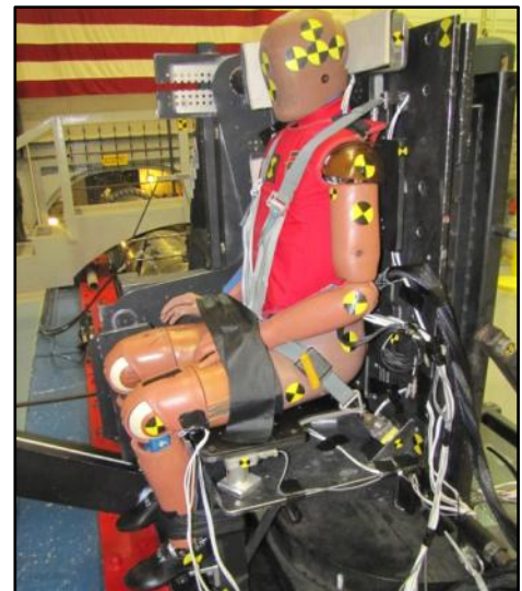
Figure 2a and 2b: HIA Facility Set-up for Lateral +Y-axis Impact Test
