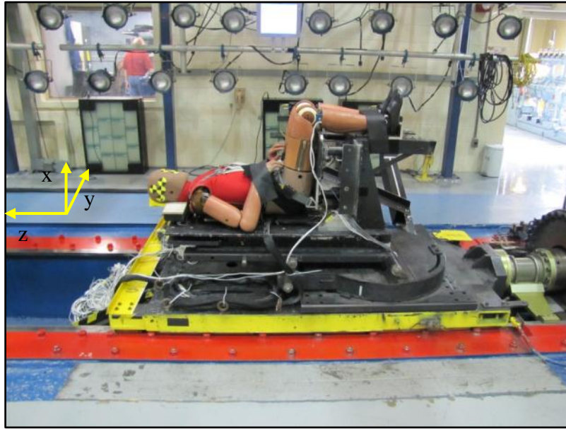
Figure 1: HIA Facility Set-up for +Z-axis Impact Test
