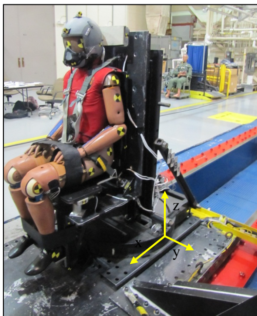
Figure 3: HIA Facility Set-up for -X -axis Impact Test
