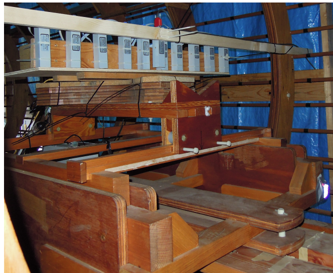
Figure 7.2: Array of Bartington MAG3-SM sensors used to measure field uniformity.
