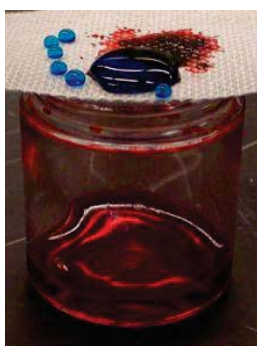
Superhydrophobic/oleophilic dip-coated fabric Tuteja et al , Science, 2007 , 318, 1618
