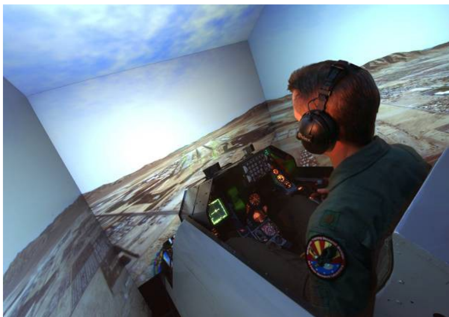
Figure 1. High Fidelity F-16 Block 30 Cockpit with M2DART Immersive Visual Display.
