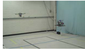
MIT/ Boeing demo - autonomous battery hotswapping on UAV
