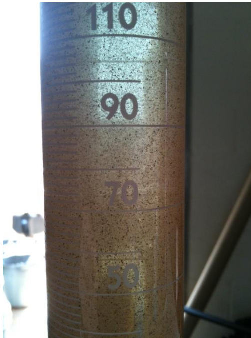
Figure 18. Close-up photograph of graduated cylinder containing boron-nanoparticle, JP-5 fuel slurry at \sim 2.5\% loading during settling experiment.
