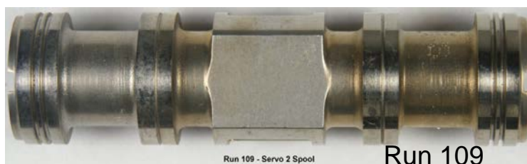
Figure H - 7 Servo Valve Spool Deposition Comparison FAME-Sensitive vs Typical Jet A
