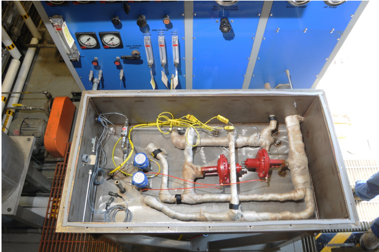
Figure 6 – Environmental Chamber for Simulation of Airframe Heat Loads
