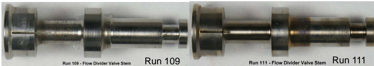
Figure H - 5 FDV Valve Stem Deposition Comparison FAME-Sensitive vs Typical Jet A
