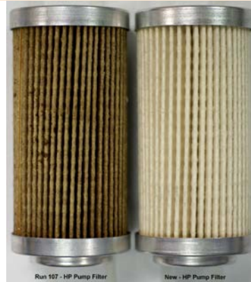
Figure G-2 – HP Pump Filter Comparison, EDTST Protocol, HT+ Conditions
