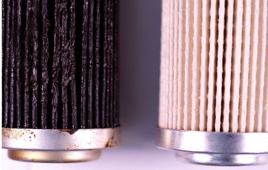
Figure 16 – Comparison of Post-Run 102 Filter and a New Filter
