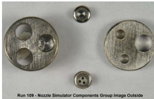
Figure H - 8 Nozzle Screen Deposition Comparison FAME-Sensitive vs Typical Jet A
