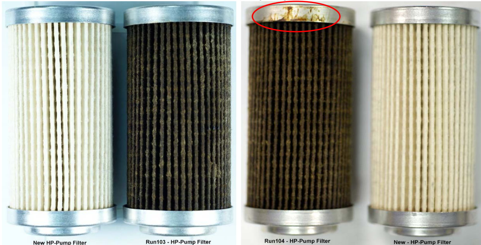
Figure G-1 - Comparison of JP Pump Filters for GDTC Runs 103 (Baseline, HT) and 104 (FAME, HT)
