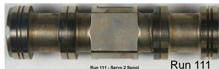
Figure H - 7 Servo Valve Spool Deposition Comparison FAME-Sensitive vs Typical Jet A
