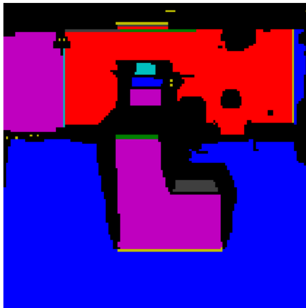
Figure 4. Planar region detection of Odette range image. Non-connected colors are independent planar regions.
