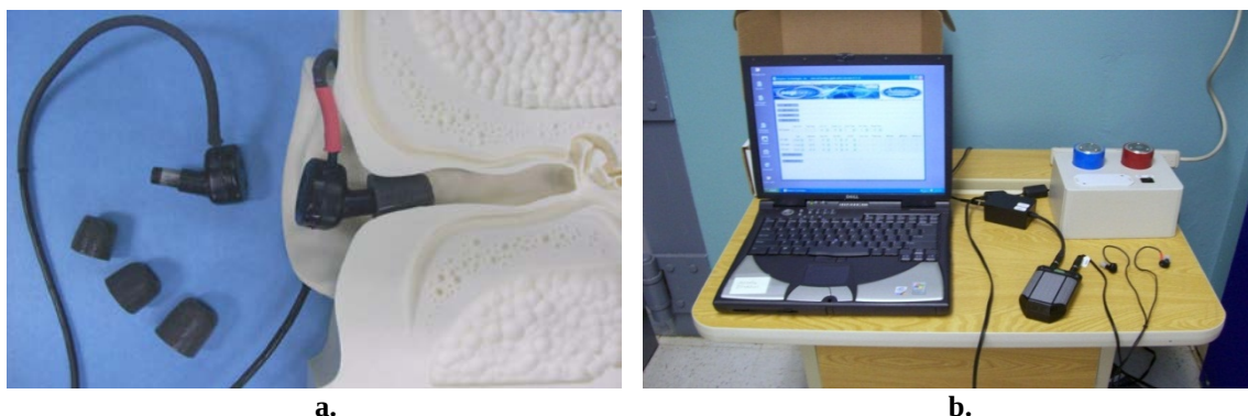
Figure 3. a. ATI non-custom earplugs b. In-ear dosimeter, calibration device, and analysis equipment
