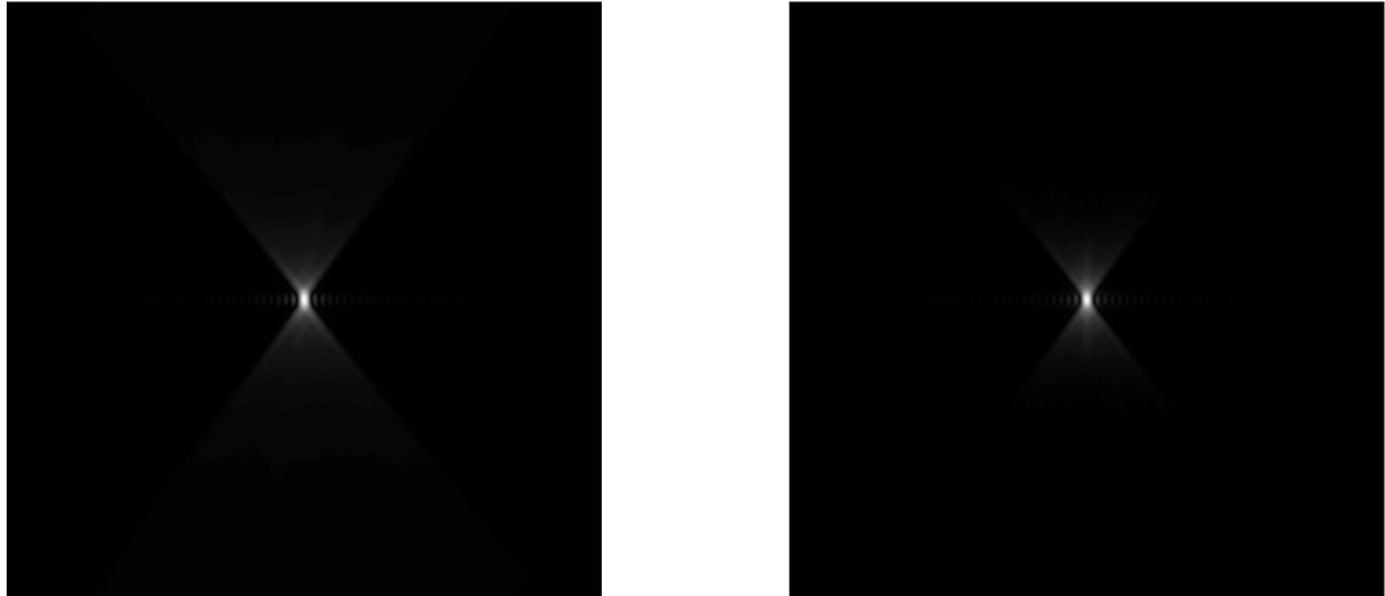
Figure 47: Fourier transform of PSF (left) and the object focal stack (right)
