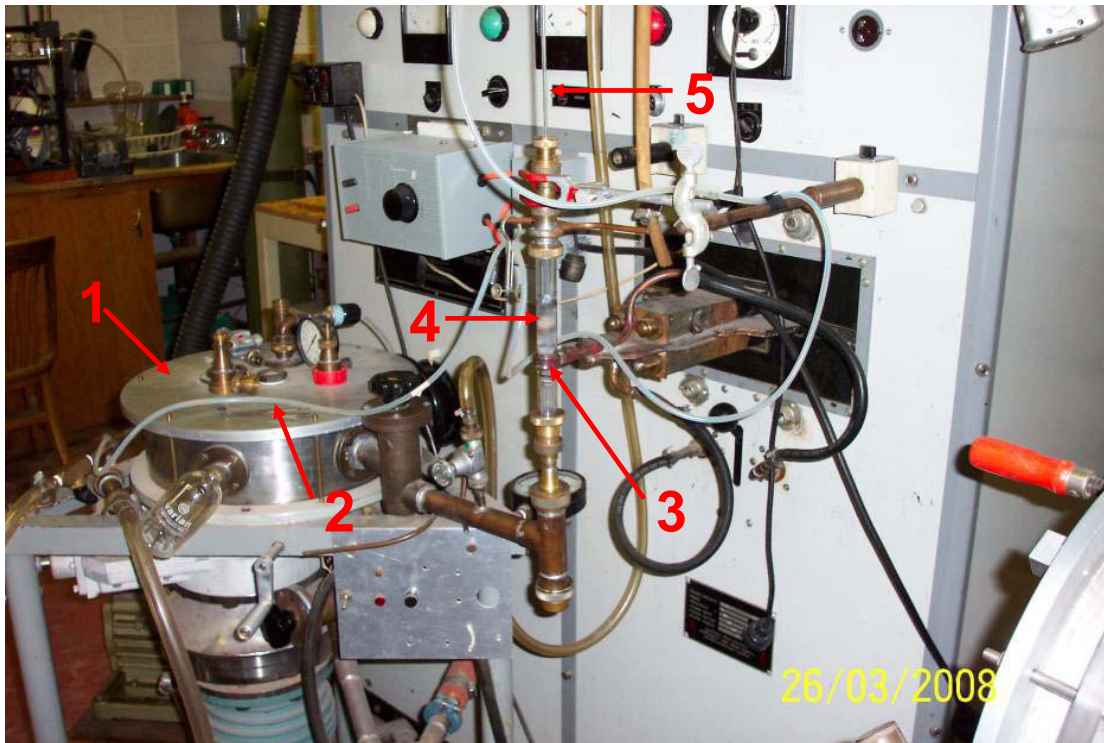
Figure 2: Photograph of the suction casting apparatus; (1) vacuum pump, (2) plastic suction hose, (3) induction coil, (4) outer quartz tube and (5) quartz suction tube.
