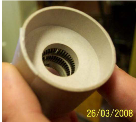
Figure 6: Zone annealing furnace heater showing heating coils.
