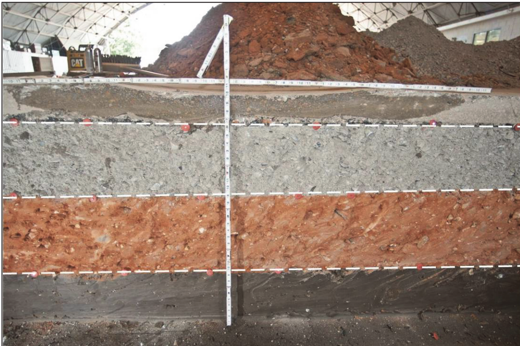
Figure 68. Foamed Asphalt North Trench (STA 0+36).
