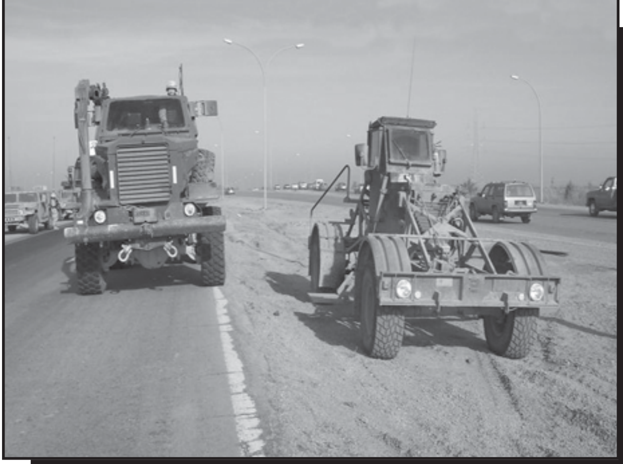
Figure 4. Buffalo (left) and Meerkat (right) Mine Detection Systems
